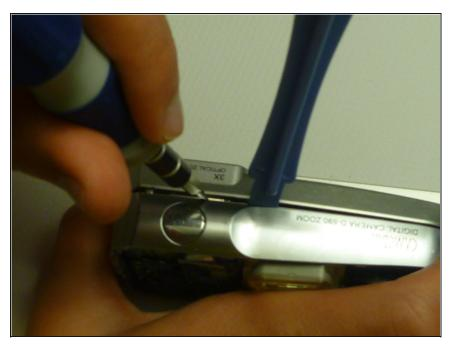
Using an iFixit opening tool, pry the backplate from the camera internal housing component.
