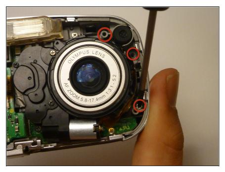
Using a Phillips #00 screwdriver, remove three screws fastened to the camera backplate edge.
