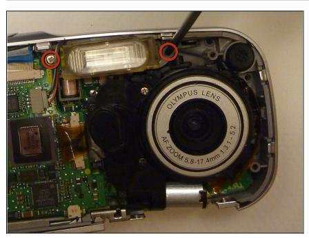
• Using a Phillips #00 screwdriver, remove the two camera flash screws secured to either side of bulb housing component.
