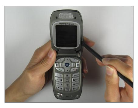
Insert a Spudger into the side crack of the flip cover and slowly separate the phone cover from the case.
