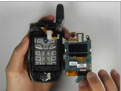
Remove the LCD board from the phone by grabbing the bottom side of the LCD board.
