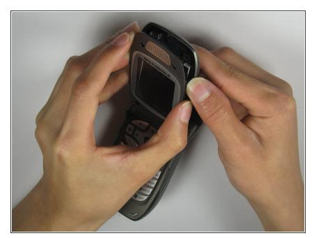
Gently separate the flip cover case from the phone with your hands when the crack is wide enough.
