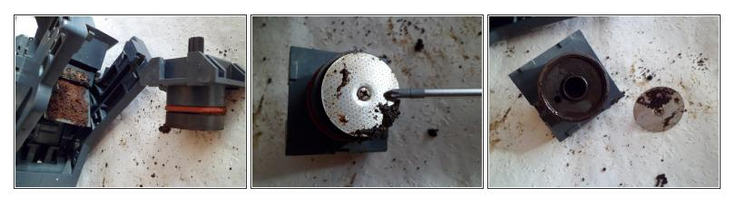
• Once the piston assembly is out, unscrew and remove the brew screen.
