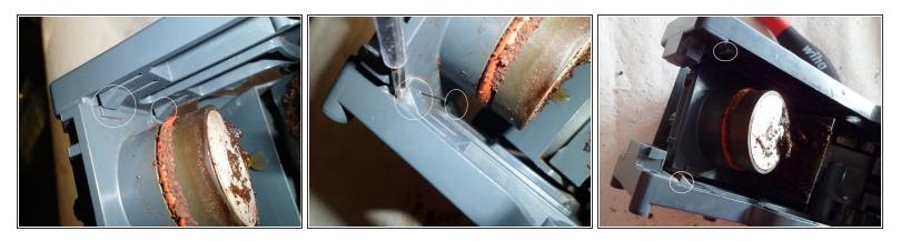
• The upper piston is held in place by four clips, two on each side. To remove it, place a screwdriver lengthwise across both clips on one side, and depress them while pushing down on the top of piston. That should loosen one side, then do the same for the other and the piston assembly should come loose.
