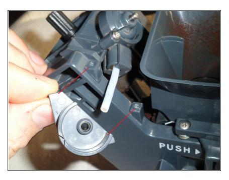
• Remove the retaining bracket.
