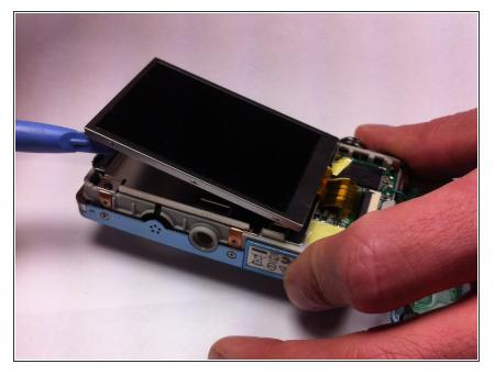
The LCD screen should now be disconnected from the rest of the camera and a pry tool can be used to lift it out of its casing.
