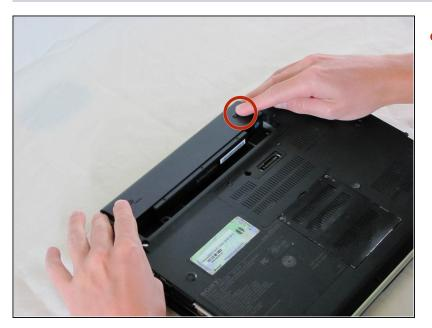
• On the opposite side of the battery, press the release latch and slide the battery away from the main body to remove.
