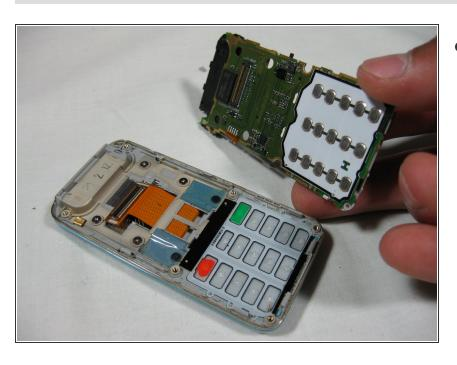
Remove the motherboard from the front casing by lifting straight up.
