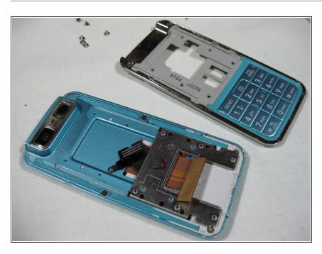
Lift the keypad housing away from the slider.
