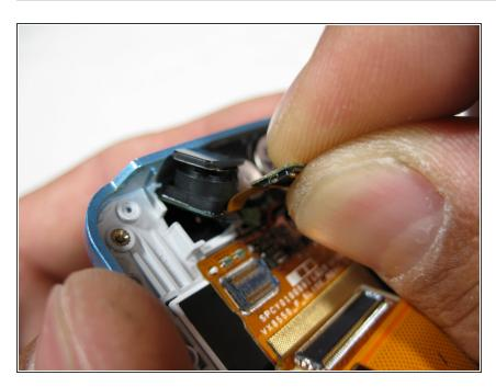
Lift up slowly on the connector cable to peel the camera off the adhesive backing.
