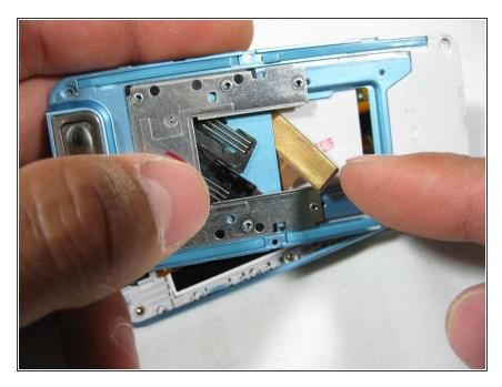
Slide ribbon cable through the slider mechanism.
