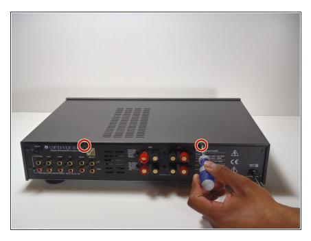
Remove 2 screws on rear of device.
