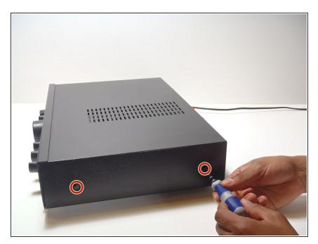
Remove 2 screws from each side of the amplifier.
