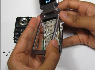
While the phone is open and faced up, carefully insert a tool into the middle to seperate the bottom half of the phone.
