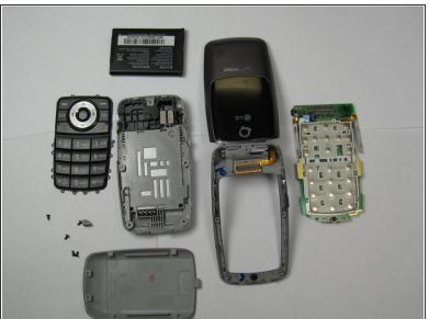
Carefully slide out the keypad and remove the logic board. Then insert new the logic board.
