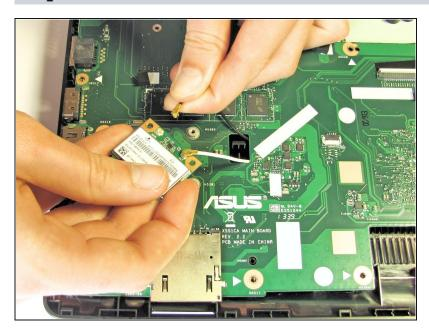
Remove each of the two small antenna connections by disconnecting one wire at a time. Each wire should easily unsnap from the Wifi card.
