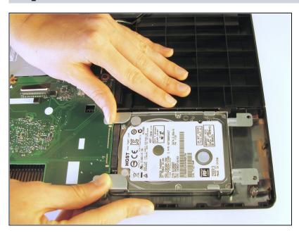
Once the screws have been removed, place your fingers on the left corners and push the hard drive towards the right edge of the laptop (relative to the picture).
