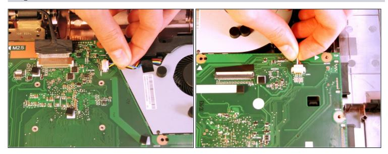
• Remove the wires by easily pulling them parallel to the motherboard's surface.
