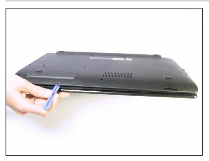
Use the plastic opening tool to separate the keyboard plate cover from the bottom cover.
