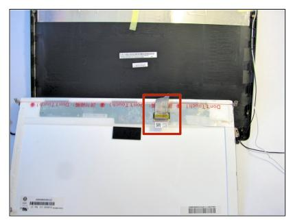
Once flipped over, locate the ribbon that is connected to the back of the LCD.
