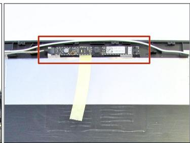
• Locate the camera on the back bezel.
