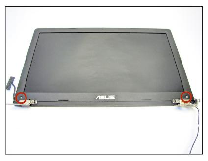
Once the stickers are removed, the two screws that hold the front bezel in place will be exposed.
