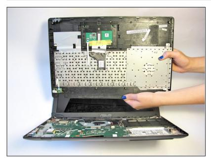
Now that the ribbons have been detached from the bottom cover, carefully remove the keyboard plate cover. Once it has been removed, place it in a safe and moisture free area so it does not get damaged.
