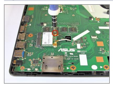
Use the Phillips #0 Screwdriver to unscrew the 3.2 mm Phillips #0 screw which attaches the WiFi card to the motherboard.
