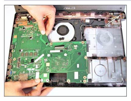
Remove the motherboard from the case by gently lifting it upward.
