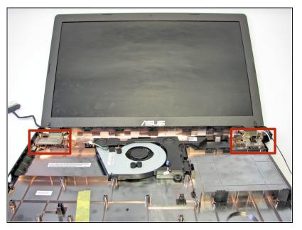
Locate both of the hinges that connect the monitor to the bottom plate cover.
