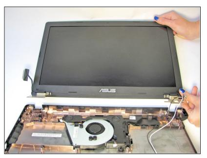
Once the screws are removed, the monitor should easily lift away from the bottom plate cover
