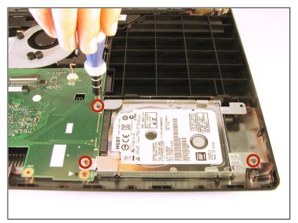
Unscrew the three 5.5 mm Phillips #0 screws with the Phillips #0 Screwdriver.
