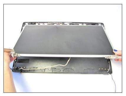
Once the screws are removed, lift up the LCD to expose the wire connecting the back bezel to the LCD.
