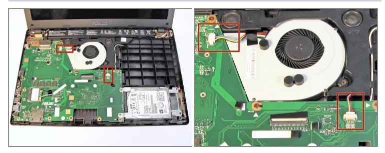
Now, locate the two wires connected to the motherboard.
