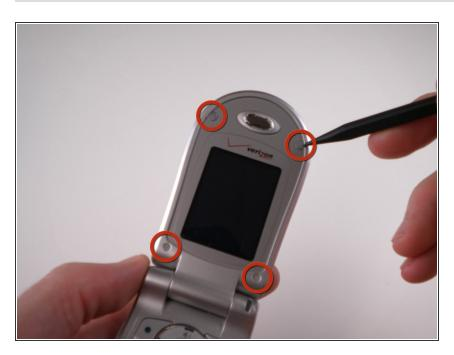
Remove 4 rubber grommets using the Spudger.
