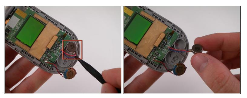
Remove vibrator using the Spudger.
