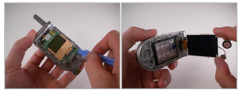
Lift up LCD display using iPod Opening Tool.
