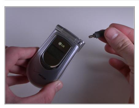
• Twist antenna counter-clockwise until detached.
