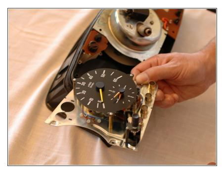
You will now be able to carefully lift the tachometer/clock assembly out of the cluster. Set it aside someplace safe. Do not set it face down, on the needles.
