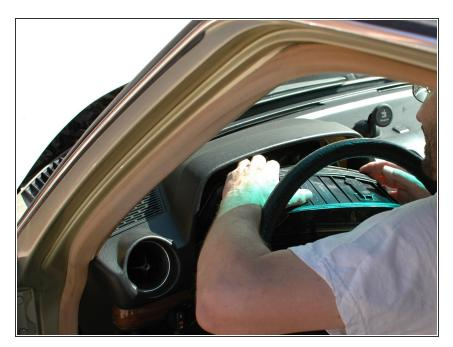
You'll need to begin by removing the instrument cluster from the car. You can read the removal guide for this process if you need help with this.
