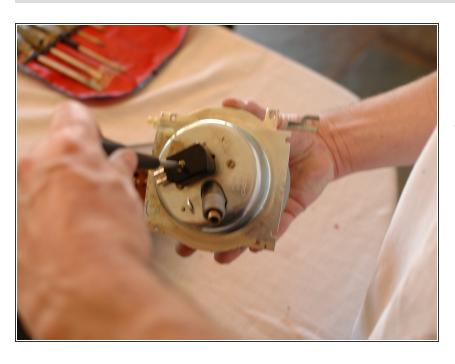
Now, remove the single screw that holds the black plug on the back of the speedometer assembly. With the screw removed the plug pulls out of a slot.
