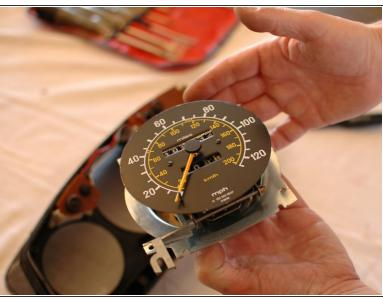
You can now lift the speedometer assembly out, carefully. Note that there are wires that cross behind the gauge face; you will need to clear these wires to remove the gauge.
