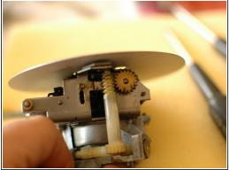
Removing the metal cover will expose the odometer. Inspect the various plastic gears for broken parts. If you find any, they will need to be fixed before continuing.
