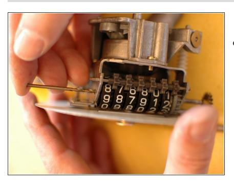
As soon as the metal shaft with the brass gear becomes loose, chase it out with an appropriately sized drill bit. Go slowly to make sure you don't leave too much space between the shaft and the bit or else one of the numbers might fall out of alignment.
