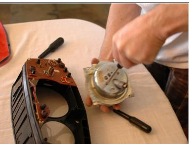
Now you can remove the two flat head screws that hold the metal back on the speedometer assembly.
