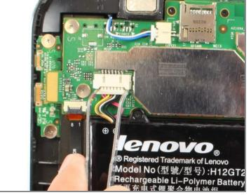
• Disconnect battery power connector by pinching the connector with <u>tweezers</u>, and sliding it out of the housing.
