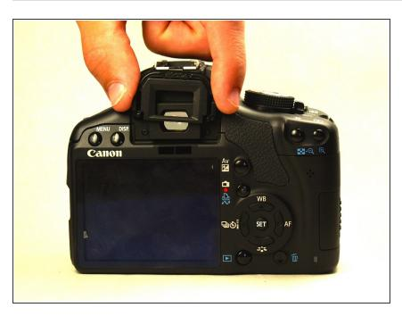
Pinch your fingers together and wiggle the eye piece gently upwards until it is detached from the camera. To reassemble your device, follow these instructions in reverse order.
