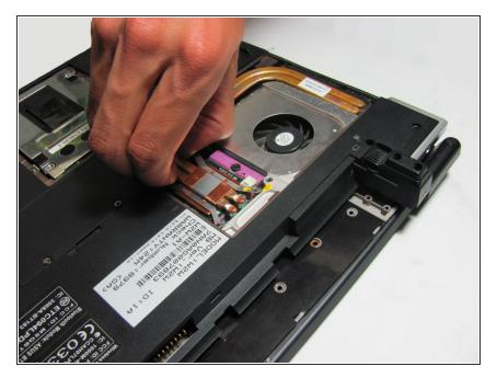
• Gently lift the orange cooling system upward to remove it from the laptop.
