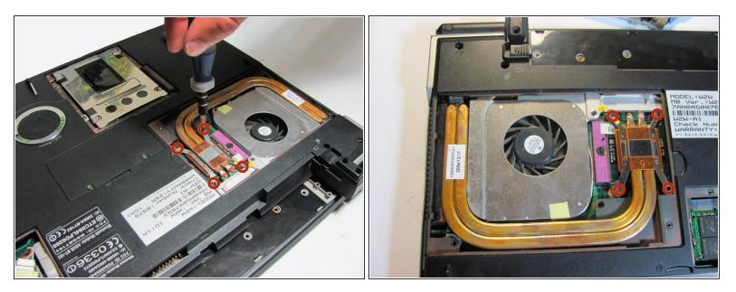
Remove the 4 4 mm Phillips screws on the orange cooling system.
