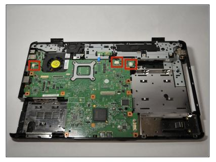
Disconnect the Thermal Fan cable, Speaker cable, and USB Board cable from their connectors.
