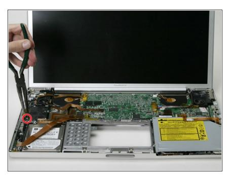
Remove the three 4 mm hex nuts using a nut driver or needle-nosed pliers.
