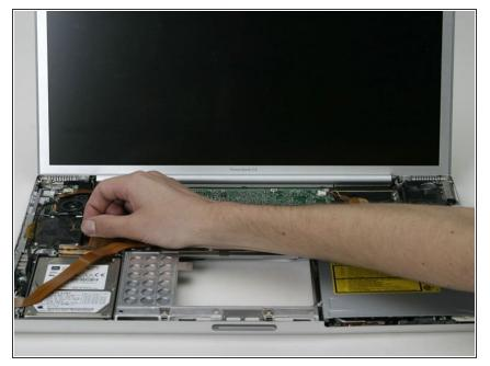
• Disconnect the orange ribbon from the right side of the modem, removing tape as necessary.
