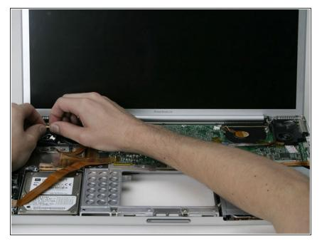
Back inside the computer, disconnect the Airport antenna cable at the gold connector, making sure you pull only on the gold metal portion of the connector.
