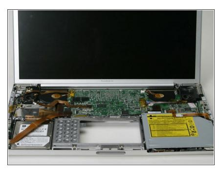
If you have not already done so, disconnect the hard drive ribbon and PC card cage ribbon from the left side of the logic board.
