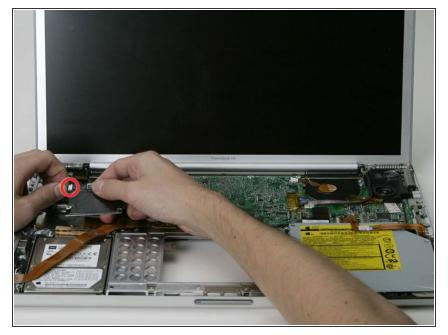
• Lift the modem partially out of the computer, disconnecting the modem cable before pulling it entirely away.
