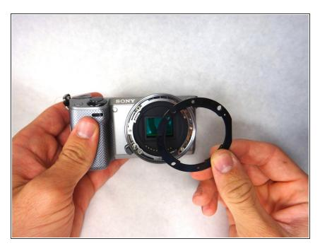
Now the black plate should be exposed. You can remove this again by gently pinching with your fingers and lifting up.
