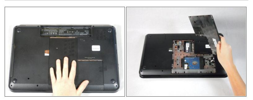
• Slide the back panel down and pull it up.
