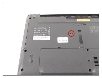
Turn the computer over and locate the screw that is in between the battery and cover panel as shown in the picture.
