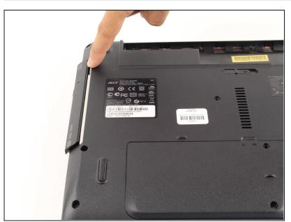
• Carefully pry the optical drive loose.
