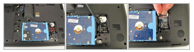
Using a spudger, disconnect the hard drive connecting cable. Use a slow, prying motion as if pulling a nail out of wood.
