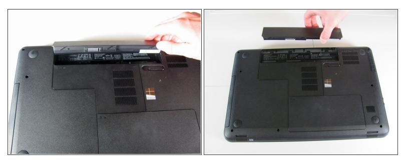
Slowly pull the battery out of its slot, being careful not to damage any of the connectors in the process.
