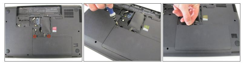
• Loosen the two Phillips #00 screws that are securing the hard drive compartment.
