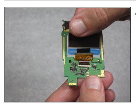
Using your fingers, carefully pull out the small LCD display screen.
