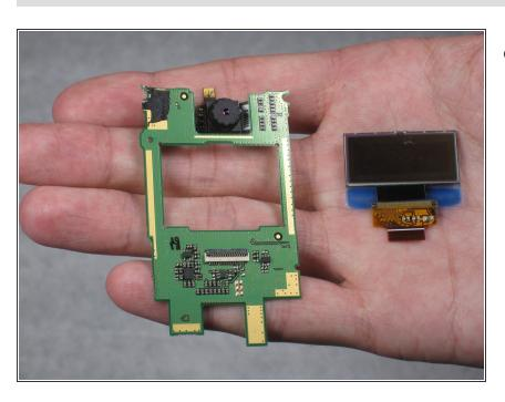
Remove the small LCD display screen completely from the green logic board.
