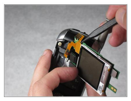
Use Spudger or hands to detach flex cable from front screen logic board
