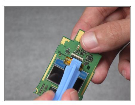
Use a plastic opening tool to lift the small black flap to unlock the screen from the motherboard.
