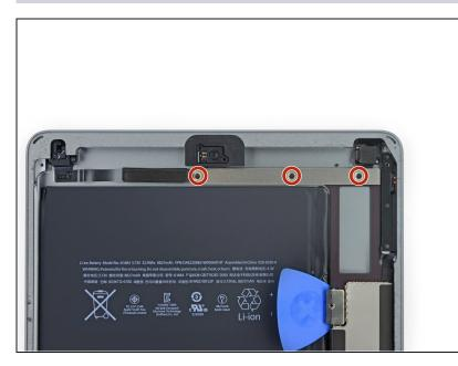
Remove the three 1.4 mm Phillips #000 screws securing the upper component cable bracket.
