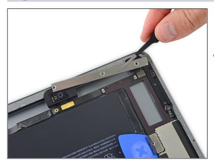
• Remove the upper component cable bracket.
