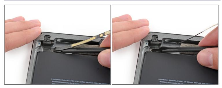
• Continue to slide the spudger under the end of the headphone jack cable to remove the last of the adhesive.
