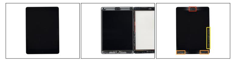
(i) While the iPad looks uniform from the outside, there are delicate components under the front glass. To avoid damage, **only** heat and pry in the areas described in each step.
