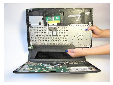
Now that the ribbons have been detached from the bottom cover, carefully remove the keyboard plate cover. Once it has been removed, place it in a safe and moisture free area so it does not get damaged.
