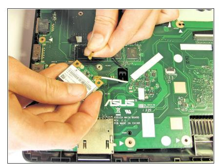
Remove each of the two small antenna connections by disconnecting one wire at a time.
