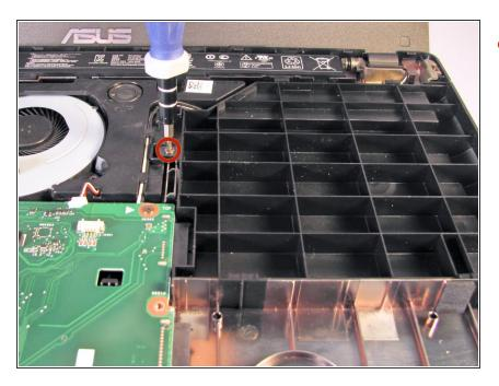
Using the Phillips #0 Screwdriver, unscrew the 5.5 mm Phillips #0 screw that holds the spacer in place.
