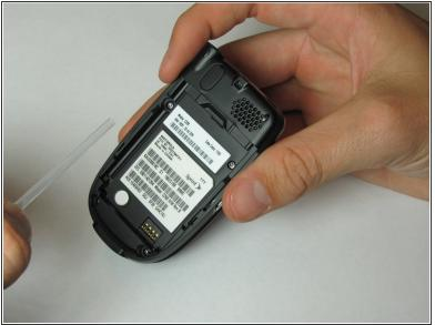
Remove the plastic tube by lifting the bottom and pulling out towards yourself.
