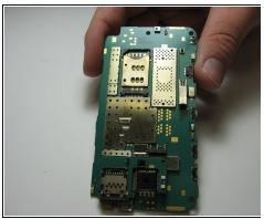
Using the blue opening tool, pry out the green motherboard.
