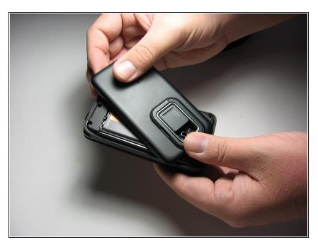
Next, locate the slit on the side of the phone and remove the back cover.
