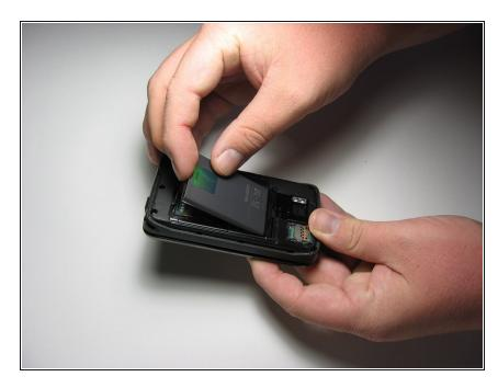
Once the back has been removed, take out the battery.
