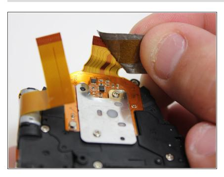
To place new lens, peel off silver tape before inserting ribbon cable into proper slot.
