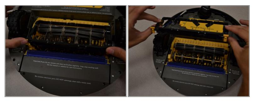
• After the guard hinges up, lift the guard up and away from the Roomba.
