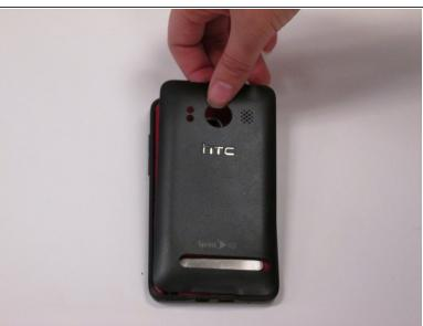
Remove the back case of the phone with a plastic opening tool by placing the tool in the tab on the back of the phone.
