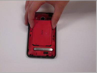
Remove the battery from the phone by carefully lifting it out with your fingers.
