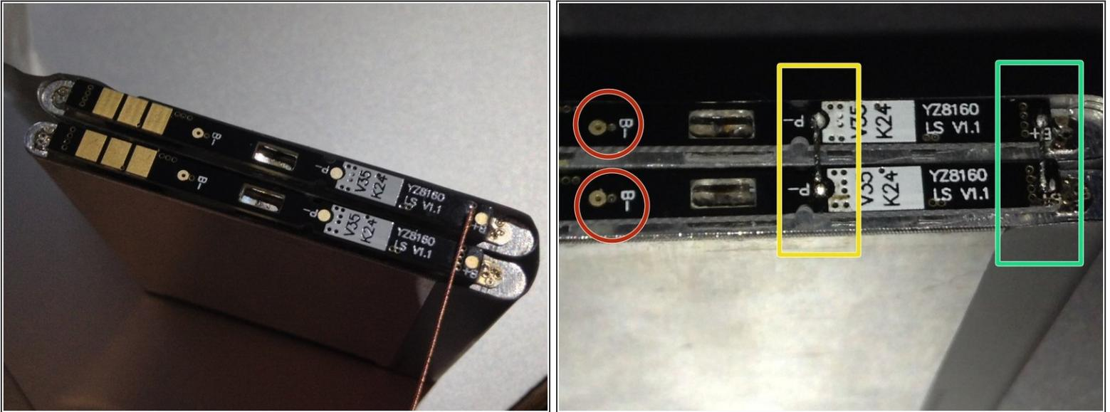
**⚠ Before bridge 2 batteries together, ensure voltage difference between them less than 50mV. New batteries will very likely have about 3.9V voltage, and varies very little.**
