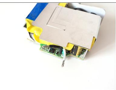
Using a utility knife or wire cutters, expose and prep the 4 wires like so.
