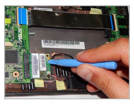
Remove the wifi antenna connection using the plastic opening tool.
