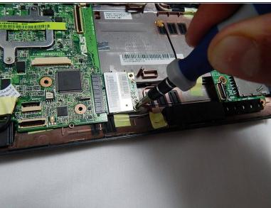
Remove this screw, which holds the wifi component in place, using the Phillips head screwdriver.
