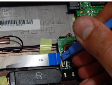
Lift the black clips using the plastic opening tool to detach the ribbon that connects the SD card module.
