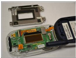
Use the pry bar to lift the metal cover from the screen housing.
