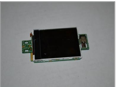
Remove the screen from the front panel of the device.
