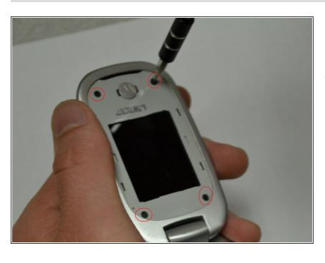
Using the T6 tool, remove the four 5mm screws on the face of the display (circled in red). Before replacing the screen, the four screws beneath the display must already be removed.
