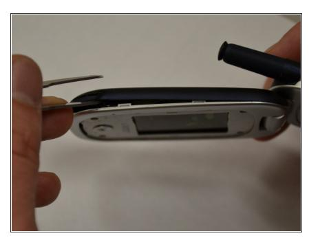
Insert the tweezers between the front and back panels of the top half of the device. Make as large a gap as possible using the tweezers.
