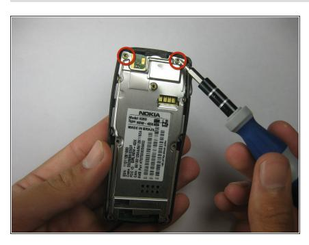
Remove the two screws at the top.
