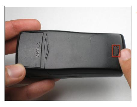
Press down on the round button on the back cover of the phone.
