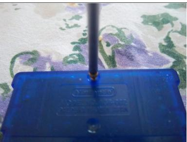
Use a Y1 screw driver to remove the screw on the back of the game cartridge.
