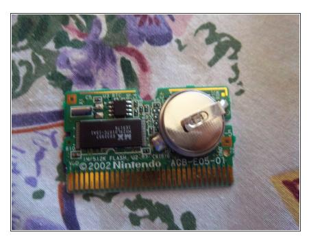
Place the new CR1616 battery in between the two contacts with the positive terminal facing down (textured side up).
