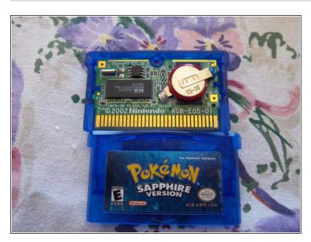
Place the ROM board into the bottom cartridge casing. Replace the top casing and the Y1 screw.
