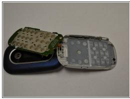
Using the plastic opening tool, gently lift the circuit board off of the four gray pegs that it rests upon.
