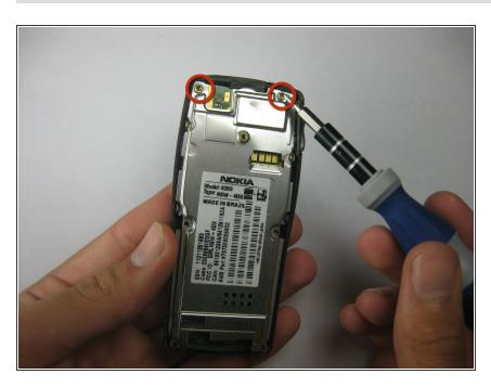
Remove the two screws at the top.
