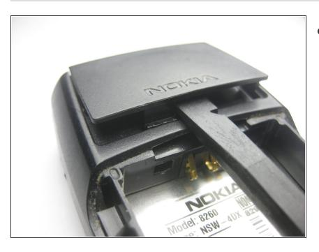
Pry open the antenna door by pulling down the top of the spudger
