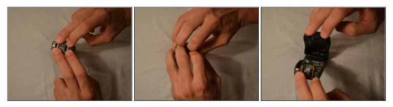
Gently open phone casing along the seam at the bottom of the phone using index and middle fingers of both hands
