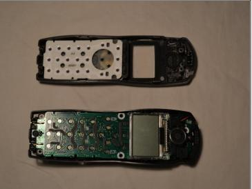
Place circuit board gently on the back shell with the earpiece facing up
