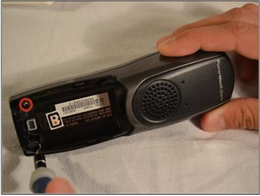
• Remove the two 11mm screws inside the battery storage compartment using Phillips #1 screwdriver (located near the very bottom of the phone)
