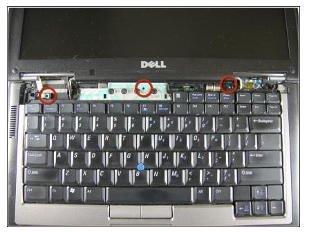
Unscrew the top portion of the keyboard using a #00 screwdriver
