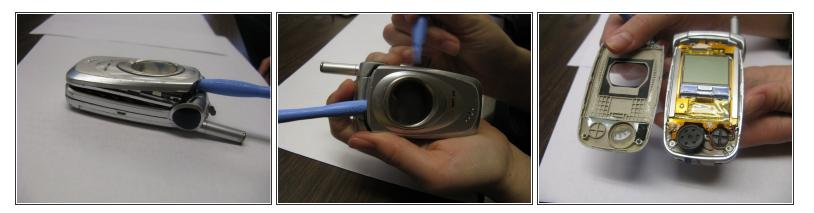
The small electronic components inside the phone are fragile; take care not to damage them when completing this step.
