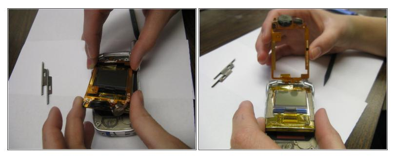
↑ The copper frame is attached to the phone at the hinge. Do not tear the frame.
