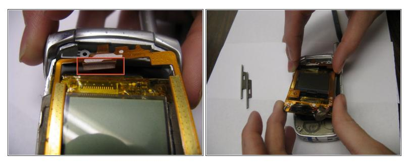
• With the copper screen lifted up, gently pull out the ribbon connector and lift out the LCD screen.
