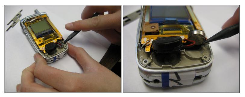
$\bigwedge$  Do not detach or tear any wires when completing this step.
