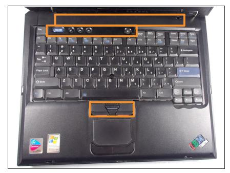
Take the spudger tool, go around the edges of the oranges boxes shown, and pop off those two sections. Then, go around the edges of the keyboard, and it should slide off.
