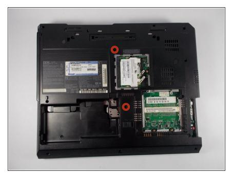
Remove the screws shown. These screws are connected to the keyboard.
