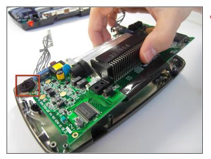
Slide the logic board out from under the circular black fastener at the top-left corner of the case.
