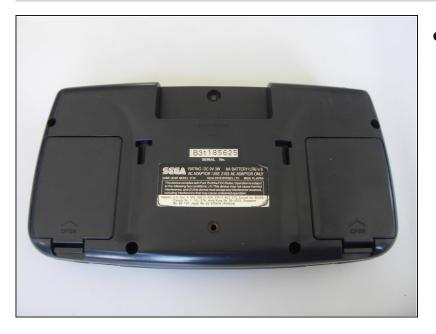
• Place your device upside down and locate the two battery compartments.
