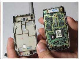
↑ Be careful when removing the casing as the spudger can damage the plastic cover of the phone.
