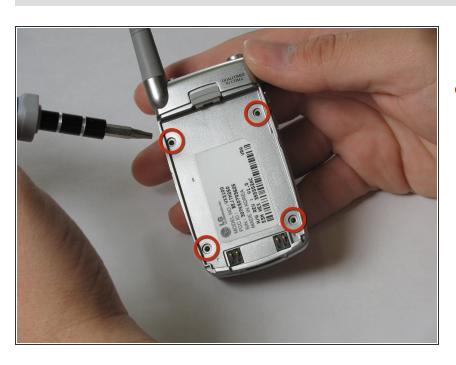
Use a T7 Torx screwdriver to remove the four screws that are located underneath the area where the battery was.
