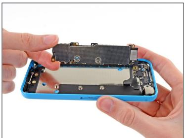
• Flip the logic board up toward the volume control buttons to expose the antenna connector.
