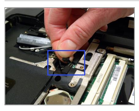
Remove the hard drive connector from the system board by lifting the Mylar tab.
