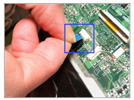
Disconnect the TouchPad cable from the system board by pulling the blue Mylar tab toward you.
