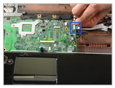
Disconnect the TouchPad cable from the system board by pulling the blue Mylar tab toward you.
