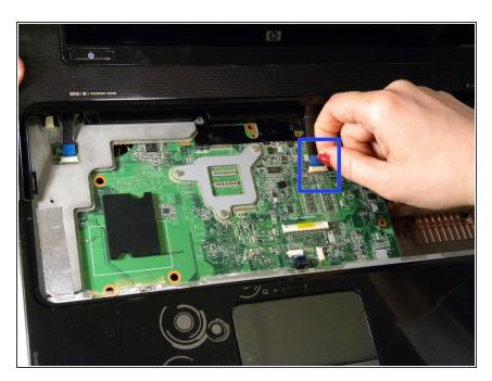
Disconnect the LED board cable from the connector on the system board by pulling the blue Mylar tab in the direction of the display (away from you).
