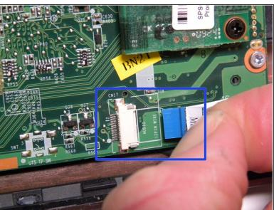
• On the side facing closest to you, pull right on the blue tab of the audio/infrared board cable to release from the connector on the system board.
