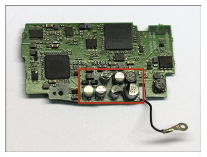
The board is now free for replacing the 6 capacitors.
