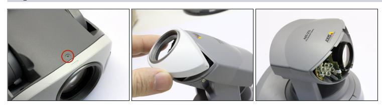
• Take out the screw under the lens. Gently tilt front upwards and remove.
