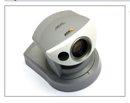
This the AXIS 213 in which the "NO VIDEO" error occurs. We will get to the 6 capacitors to be replaced.
