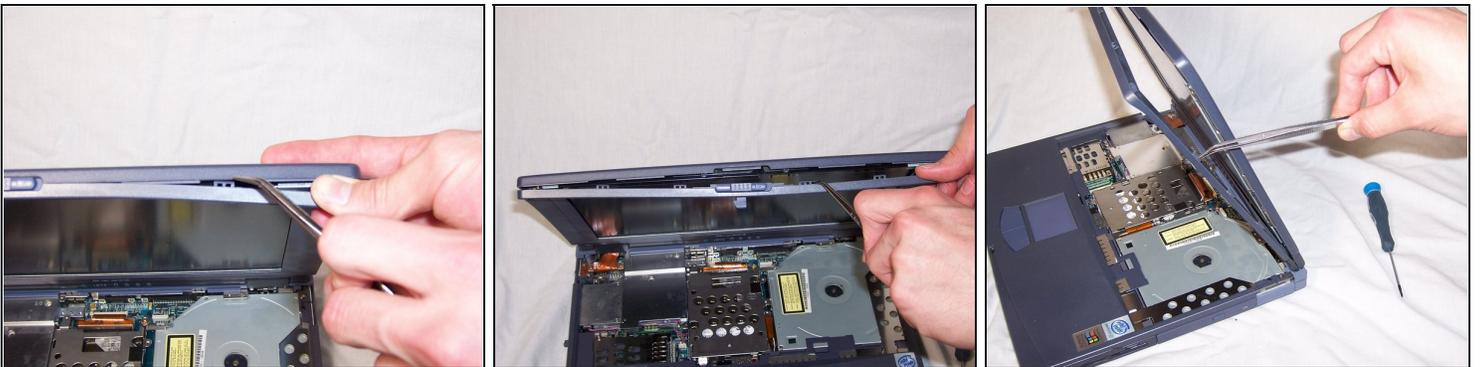
ⓘ There are a total of 14 clips holding the two bezel panels together. Be careful when unclipping all of them. After all the clips are off, the bezel will just pop right off the display panel.
