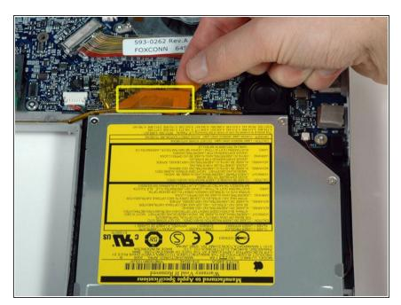
• Disconnect the orange SuperDrive ribbon cable from the logic board, removing tape as necessary.
