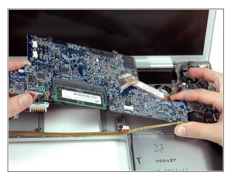
• Grasp the logic board at the left side and at the thin section near the right fan, and rotate the logic board out of the lower case.
