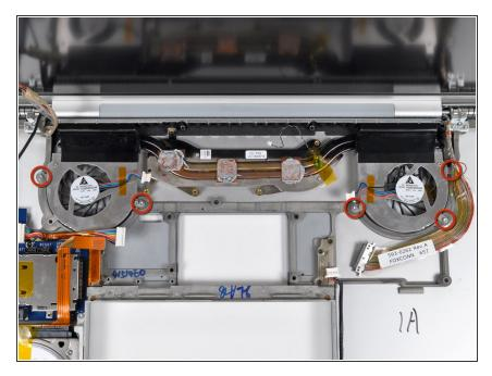
Remove the five 7.8 mm T6 Torx screws securing the fans to the lower case.
