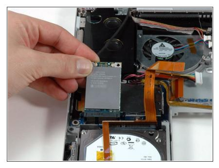
• Lift the AirPort Extreme card up and slide it out of its connector.
