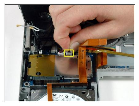
• Disconnect the right speaker from the left I/O board. Make sure to pull on the top section of the white connector, not the cable itself.
