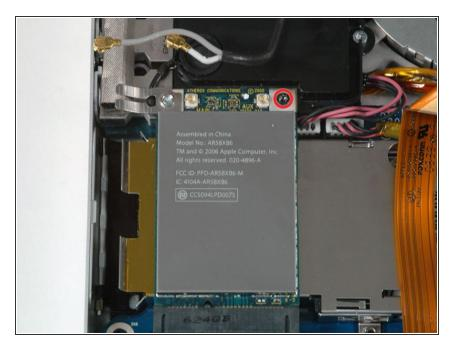
Remove the single black 4 mm T6 Torx screw from the top right corner of the AirPort Extreme card.
