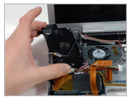
Lift up on the left speaker assembly and rotate it slightly. It is not possible to entirely remove the speaker yet, as it is still connected to the left I/O board beneath.
