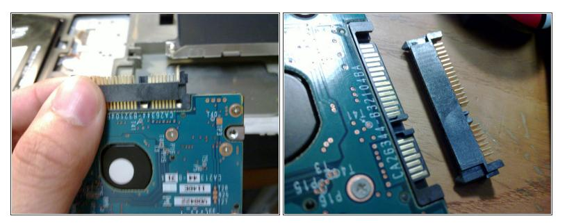
With even pressure on both sides, take off the SATA converter and then connect it to the drive you
