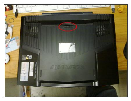
• First, take off the battery by moving the latch to the left and pulling it up.
